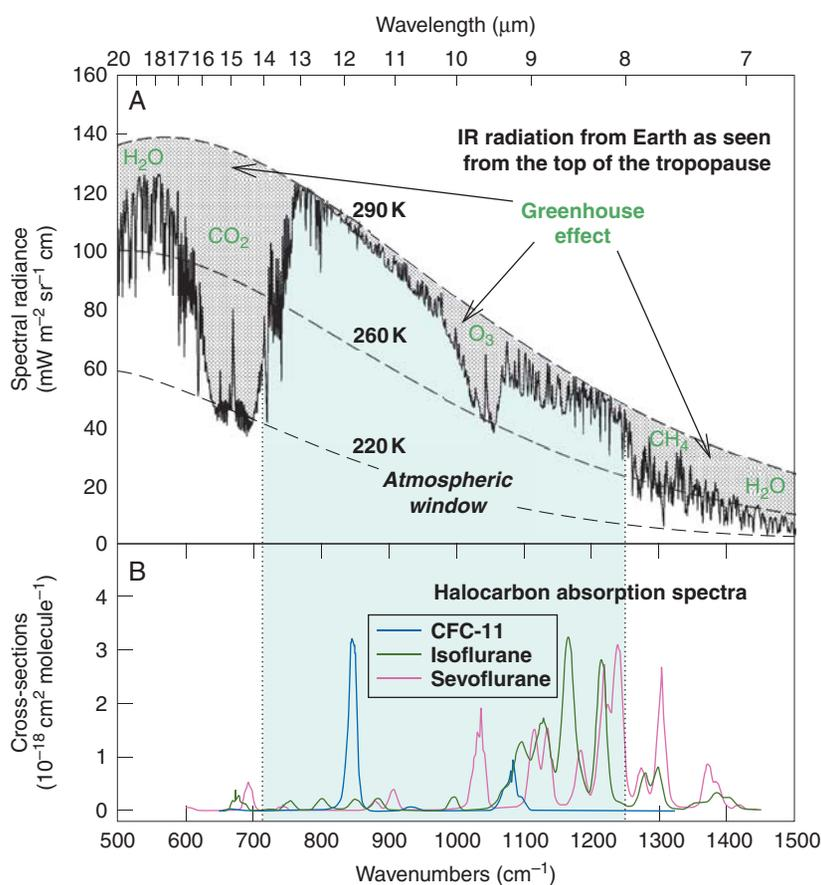
**Fig 1** (A) The net upward atmospheric radiance spectrum at the tropopause.<sup>22</sup> Dashed lines are Planck functions for blackbody emissions at 290, 260, and 220 K, respectively. (B) IR absorption bands for CFC-11 ( $\text{CCl}_3\text{F}$ ), isoflurane, and sevoflurane. Halogenated organic compounds absorb strongly in 'the atmospheric window' region.
